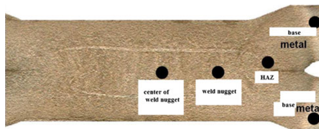
Fig. 8 Macro-structure and different regions in spot-welded sheets
